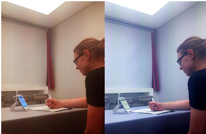
Figure 1. Room equipped with an LED luminous ceiling (Left: 2,531 K - 503 lux, Right: 19,760 K - 496 lux)
